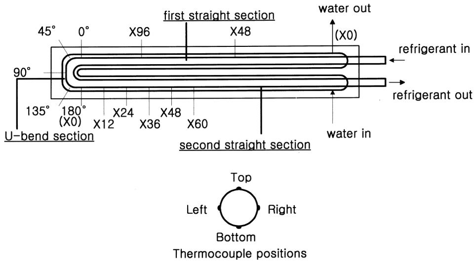
Fig. 2. Details of the test section.
