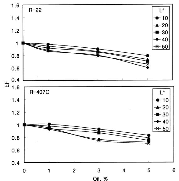
Fig. 11. Enhancement factor at each position of the second straight section for a mass flux of  $100 \text{ kg/m}^2 \text{ s}$  and inlet quality of 0.9.
