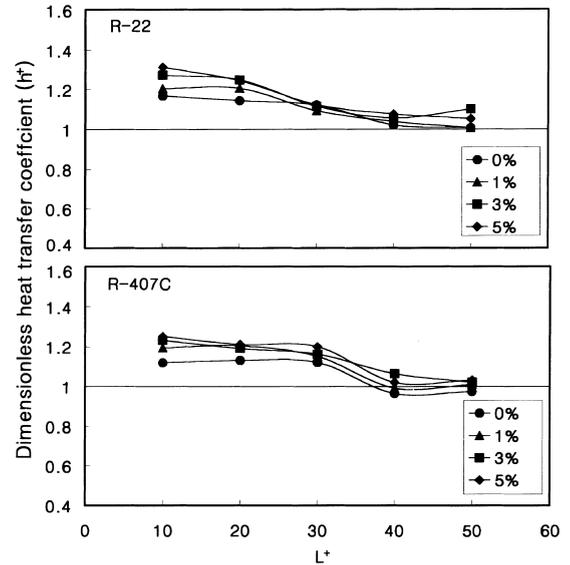
Fig. 10. Dimensionless heat transfer coefficients in the second straight section for a mass flux of  $100 \text{ kg/m}^2 \text{ s}$  and inlet quality of 0.9.
