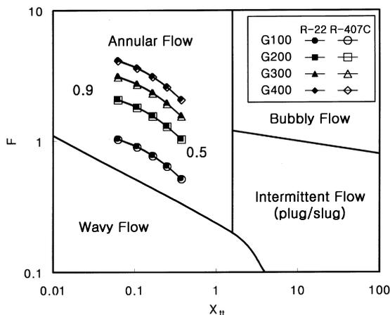
Fig. 3. Taitel and Dukler’s flow pattern map for the experimental range.
