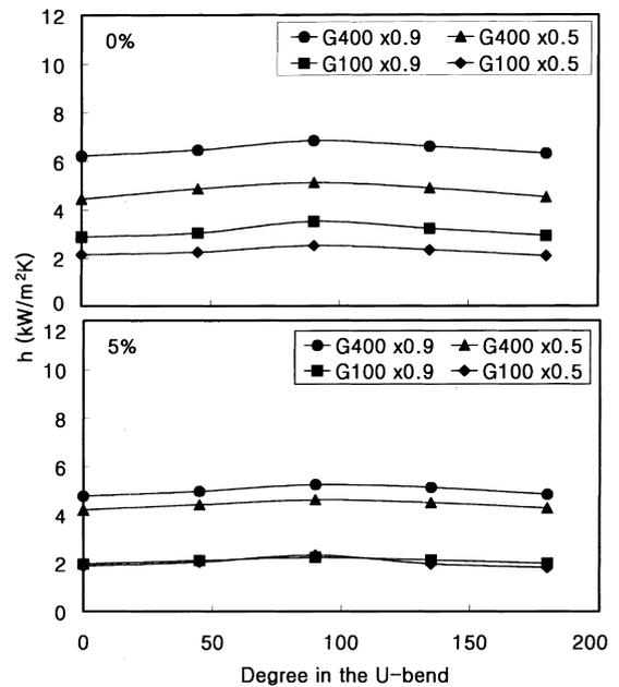
Fig. 8. Heat transfer coefficients in the U-bend section for R-407C.
