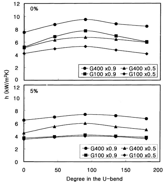
Fig. 7. Heat transfer coefficients in the U-bend section for R-22.
