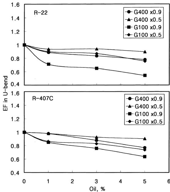
Fig. 9. EF at the 90° position of the U-bend.
