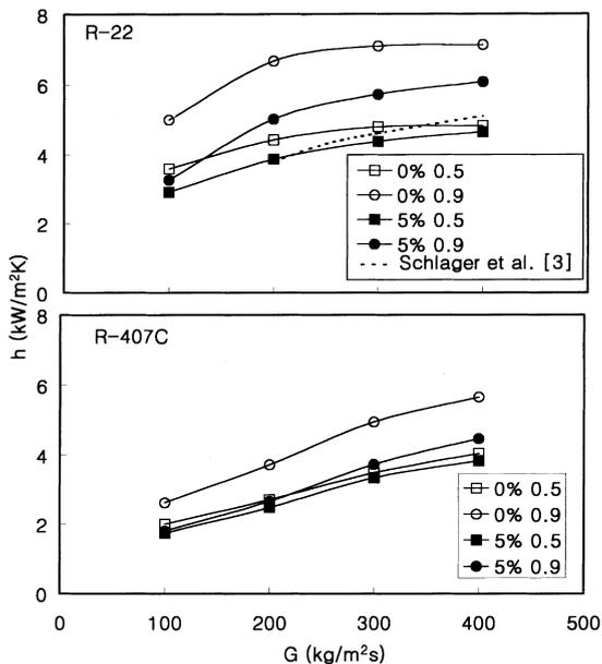
Fig. 5. Average heat transfer coefficients in the first straight section.
